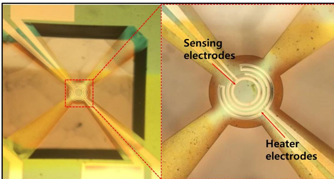
**Fig. 1** An optical image of the sensor platform. Ti/Pt electrodes (sensing and heater electrodes) are formed on the suspended SiO<sub>2</sub>/Si<sub>3</sub>N<sub>4</sub>/SiO<sub>2</sub> membrane
