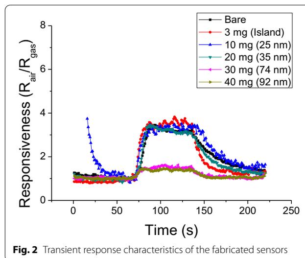
**Fig. 2** Transient response characteristics of the fabricated sensors
